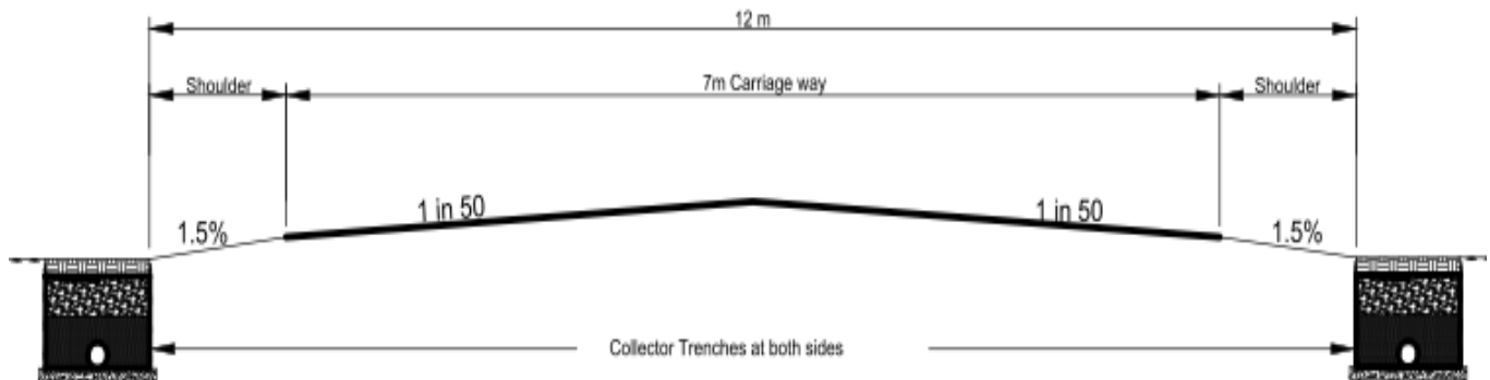
Fig. 19: Cross sectional View of Location for Collector Trench in Cutting Portion (CH:7155 to 7500)
