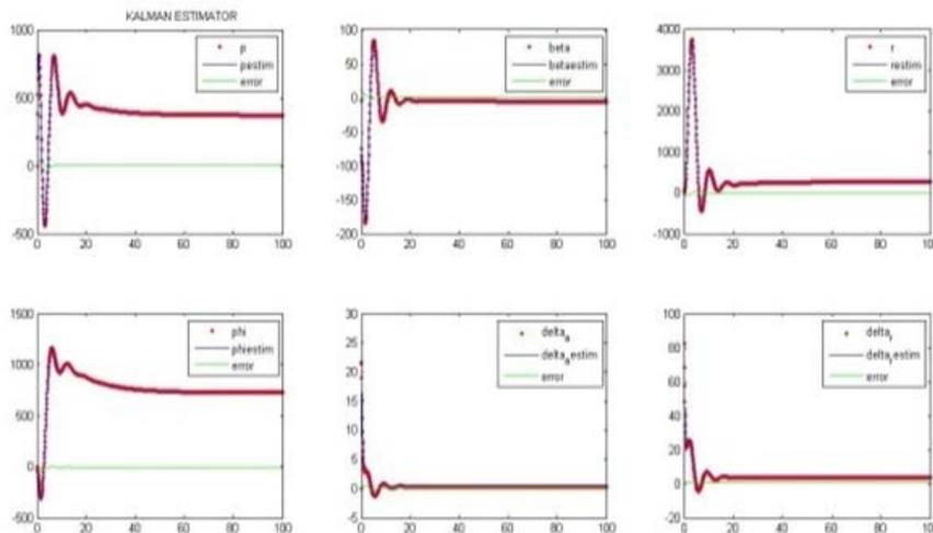
Fig. 3: Graph Indicating the Predicted, Estimated and Error Values of Lateral Parameters
