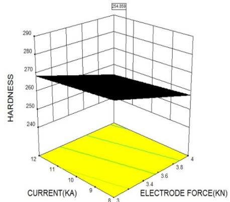
Figure 4: Weld Current Vs Electrode Force on Hardness
