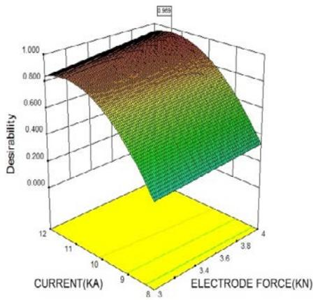
Figure 3: Weld Current Vs Electrode Force on Desirability
