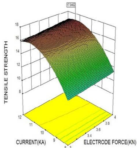
Figure 2: Weld Current Vs Electrode Force on Tensile Strength
