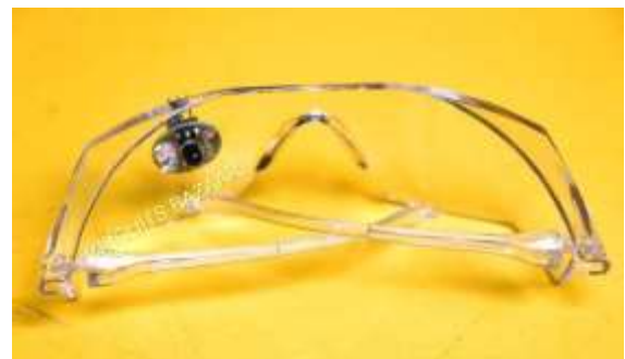
Figure 7: Goggles for Eye Blink Sensor
