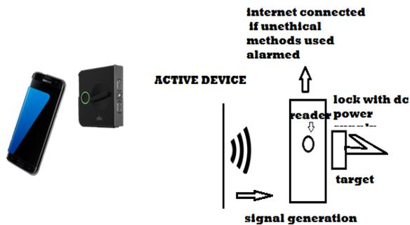
The best part of NFC tag is that it doesn't require any external power supply to operate. It gets all its energy from the field created in the course of the communication of the two devices.
